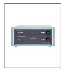
The MediBLUE automates the industry standard Methylene Blue Dye test, where packaging is submerged into a blue dye solution. The test chamber is then placed under a vacuum that forces air from any openings within the pack. After returning to an ambient pressure, the dye will penetrate and be evident within the pack should any holes be present.
